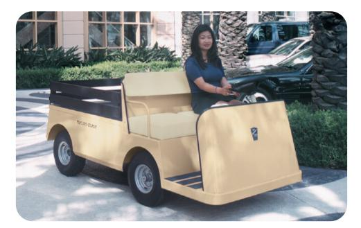
Standard equipment includes 5.70 x 8 load range B pneumatic tires, front and rear leaf spring suspension, and self-adjusting rear drum brakes, making the Carrymaster the best value in its class. Accessories include a windshield, a light package, stake sides, and utility boxes.
