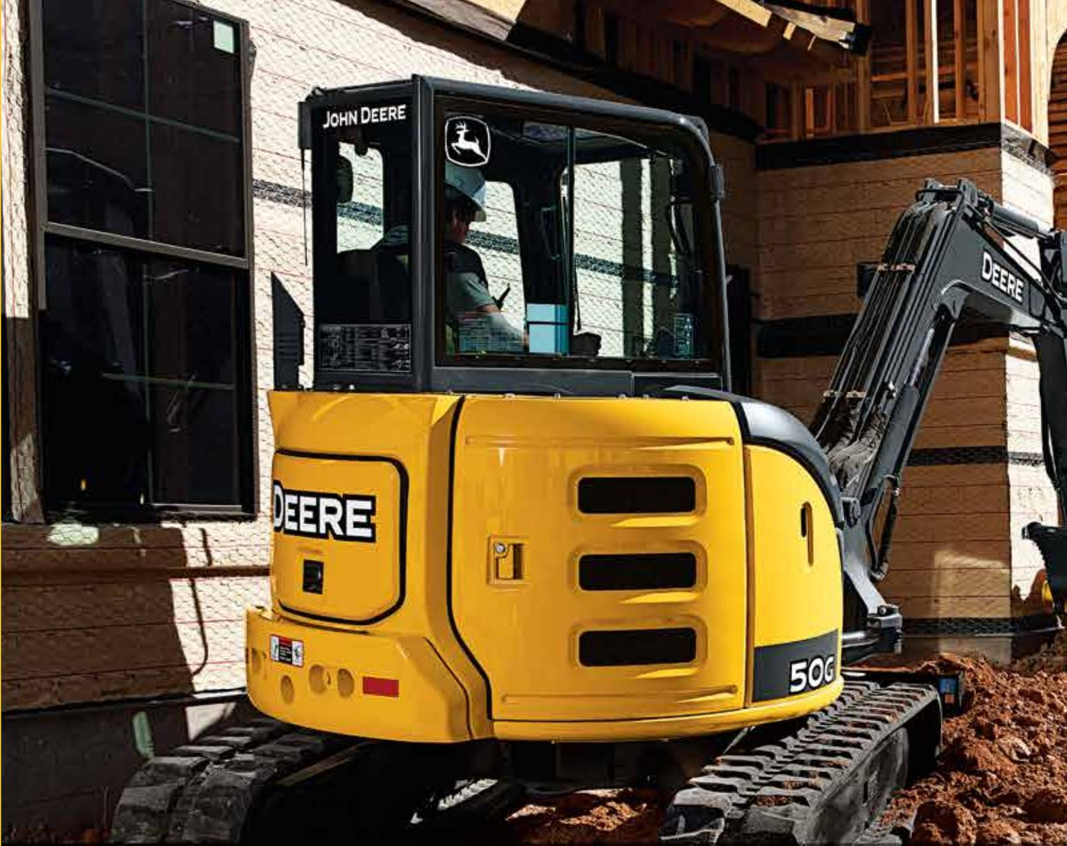
Power/economy work modes allow you to match engine speed to the application. Select **Power** mode and get the higher engine speeds needed for most general digging work. For lighter digging demands, **Economy** mode reduces engine speed and noise, while improving fuel efficiency.
